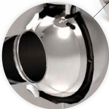
Small contact area between ball and seat for lower torques. Smaller ball to reduce pressure on seat. Better tightness at lower pressure
